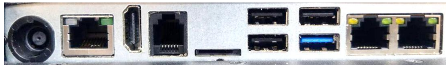
DC In 20V Giga LAN Video Port RJ-11 12V or 24V TF Card Recovery USB x2 USBx1 OTGx1 RJ-45 COM 1 RI/5V/12V RJ-45 COM 2 RI/5V/12V
